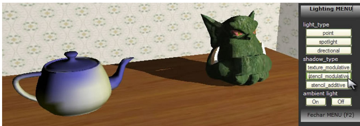
Figura 40 - Shadow Type: Stencil Modulative.
